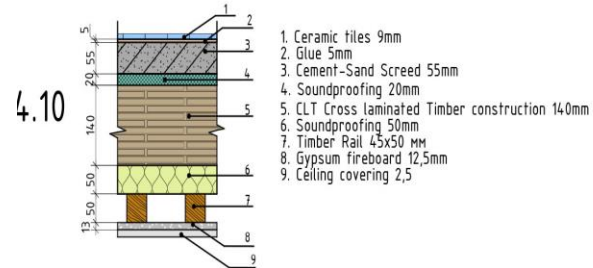
4.10 Floor construction CLT panels 140mm. Covering - Ceramic tiles.
